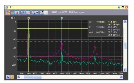
4. Viewing a real time FFT of a 1 kHz tone. The purple trace represents the peak hold channel, which shows the effect of transient conditions. The two cursors are used to measure the second harmonic level of the 1 kHz tone. In this case, the second harmonic is normally 55 dB lower than the fundamental tone; however a transient event recorded by the peak hold dramatically increased the harmonic level by approximately 25 dB.
