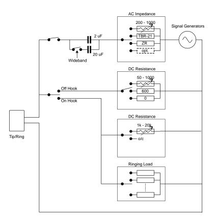
The AC impedance terminations are AC coupled to the tip/ring leads by a 2.2uF capacitor, with the option of adding an additional 20uF in parallel. This additional capacitance improves the level accuracy when generating low frequency signals. The termination impedance is selectable from either an adjustable value in range of 200 to 1000  $\Omega$ , the TBR-21 complex reference impedance, the German ZR complex reference impedance, or an optional third complex impedance (if installed).
