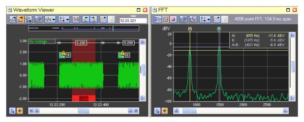
3. Viewing the FFT of a captured DTMF digit. The waveform view highlights in a red background color the time range used for the FFT calculation. Its position is always
