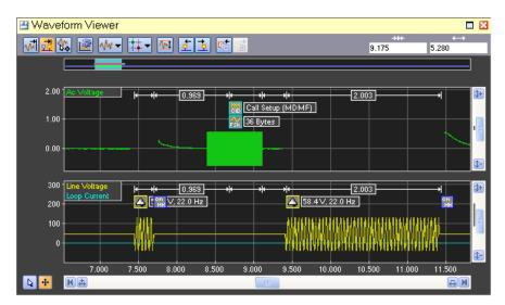
1. Capture of the waveforms present during an on-hook Caller ID transmission. The top green trace shows the AC coupled channel containing the FSK modulated data, while the bottom yellow and blue traces show the line voltage and loop current channels respectively.
