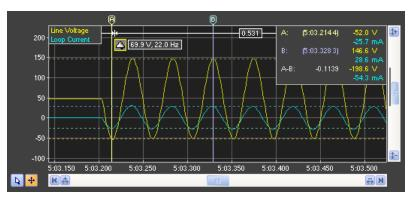
2. Capture of ringing signal with a ringing load applied. Cursors are used to measure the positive and negative peaks for both the line voltage and loop current.
