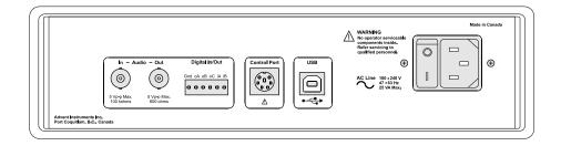
The BNC output connector can be used to monitor signals from the telephone line as well as other internal signal points. Its output impedance is 600  $\Omega$  with a maximum output level of 5 Volts peak-to-peak. The BNC input connector is AC coupled and accepts a maximum peak-to-peak signal of 5 volts. Its input impedance is 100 k $\Omega$
